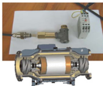
Control Unit Leakage Sensor
