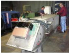
Environmentally-friendly module with internal, submersible lubricant pump and motor
