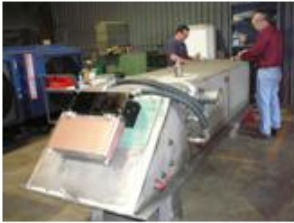
Environmentally-friendly module with internal, submersible lubricant pump and motor
